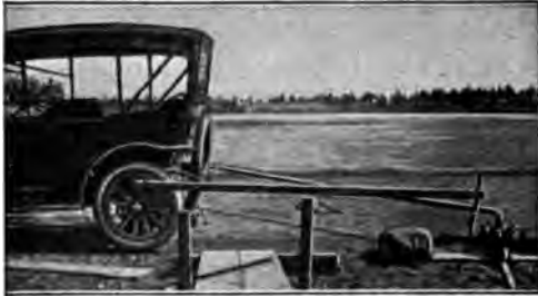
Without the Use of Pulley or Belt, the Automobile is Used to Drive a Water Pump on a Farm
